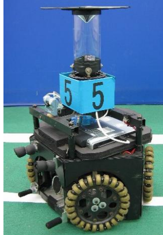
Fig. 1. Our current robot. The robot is a 4-wheeled omni-directional mobile robot with an omni-directional vision system, a normal camera and a kicking device, and is controlled by a notebook PC.
