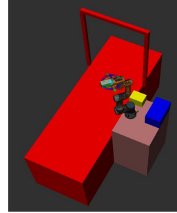
Fig. 9: The improved robot model. The blue box is an explosives detector, the yellow box is a sampling paper container and the red box is the transport belt.
