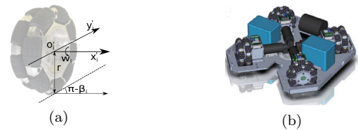
Fig. 3: Omnidirectional wheel and motion model of the wheel (a) and base frame of the real robot (b).
