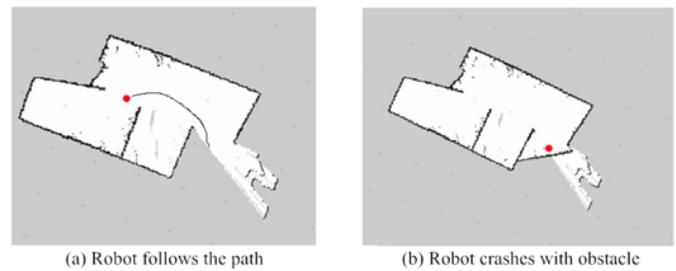
Fig. 7. A example of the robot being stuck.
